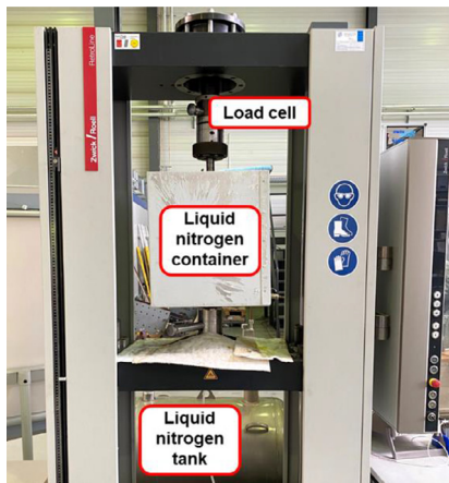
Fig. 2. Experimental setup for tensile tests at liquid nitrogen temperature.
