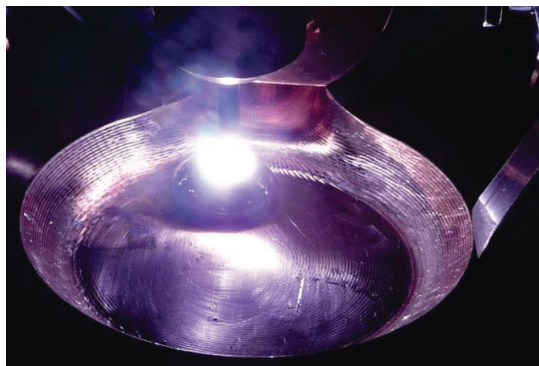
FIG. 2. (Color online) The arc-melting of a BMG alloy ingot on top of the water-cooled copper hearth. On the right is the tip of the manipulator used to flip the ingot upside-down between melting runs. The mould orifice and the melt pouring nozzle leading to it can be seen behind the electrode tip assembly.
