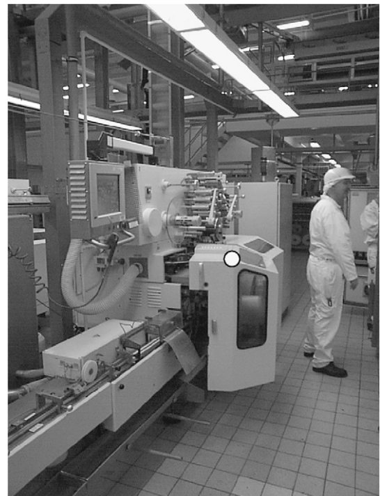
Fig. 2. Packaging machine. The dot at the top of the machine indicates a reference point for the illuminance (originally 300 lux, low-level task lighting 350 lux, high-level task lighting 2000 lux).
