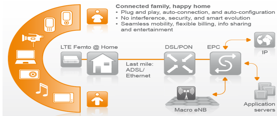
Fig. 17. Smart @ home services LTE femtocell portal
