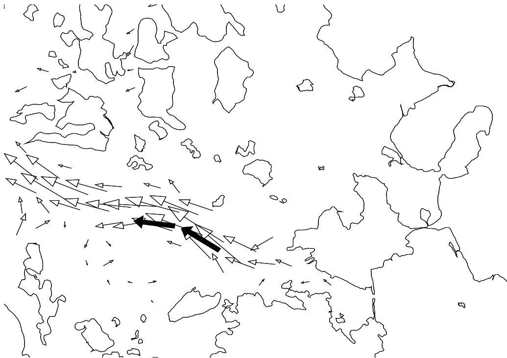
Figure 5. Flow field and calculated flows by regression equations from depth 6-8 m. Wind is 5 m/s from west.
