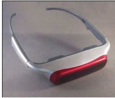
Figure 10. An example of a head-mounted display with a resolution of 640 * 480 pixels. According to the internet store in: http://www.vrealities.com/i-3d.html , where the image is from [accessed 10 Dec 2008], this device “represents a breakthrough in an affordable 3D capable Head Mounted Displays”. It is sold for $ 225 that is about 175 €.
