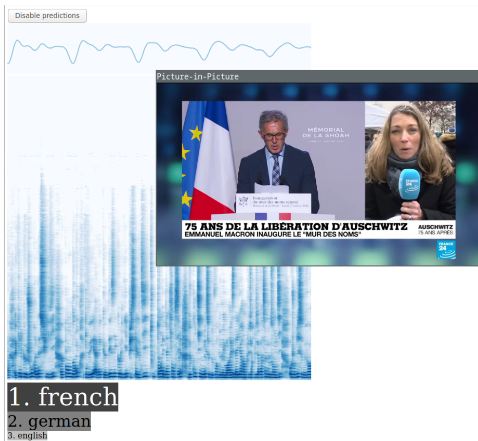
Figure 7.1. Online SLI system running in a web browser. The real-time spectrogram plot seen in the screenshot depicts a decibel-scale spectrogram of the STFT output provided by the JavaScript AnalyserNode, which is converted to model input. Here, the source audio contains speech in French, and was chosen uniformly at random from the YTN-Aalto2019 dataset.
