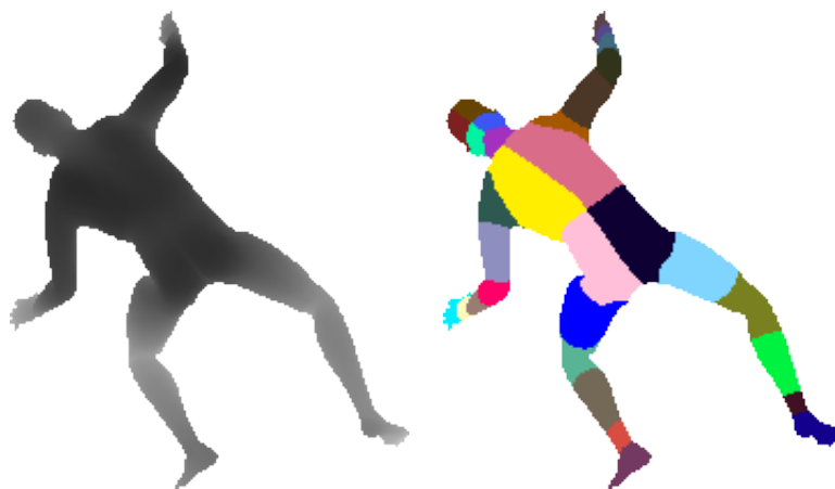
Figure 2.2: A depth image and the intermediate body part representation used in BPC
