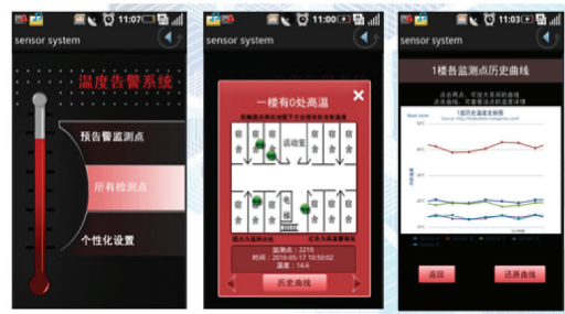
Figure 6. Temperature warning system
