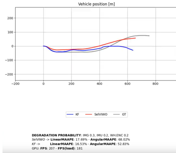
Figure 52: Dashboard comparing the methods in a section of curvy highway with degraded sensors' data.
