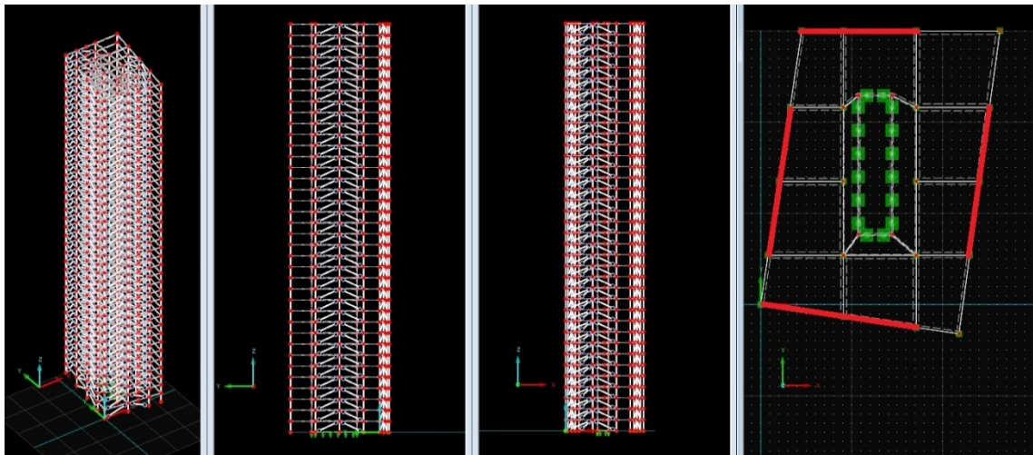
Figure 52. Finite element model with added truss system
