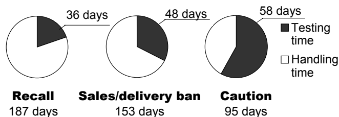
Figure 8. Segmentation of safety case durations by different measures (presented durations are mean values)
