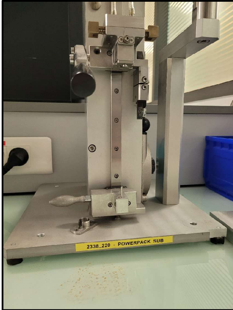
Figure 30 : Tool to remove the RiTC from the plastic parts.
