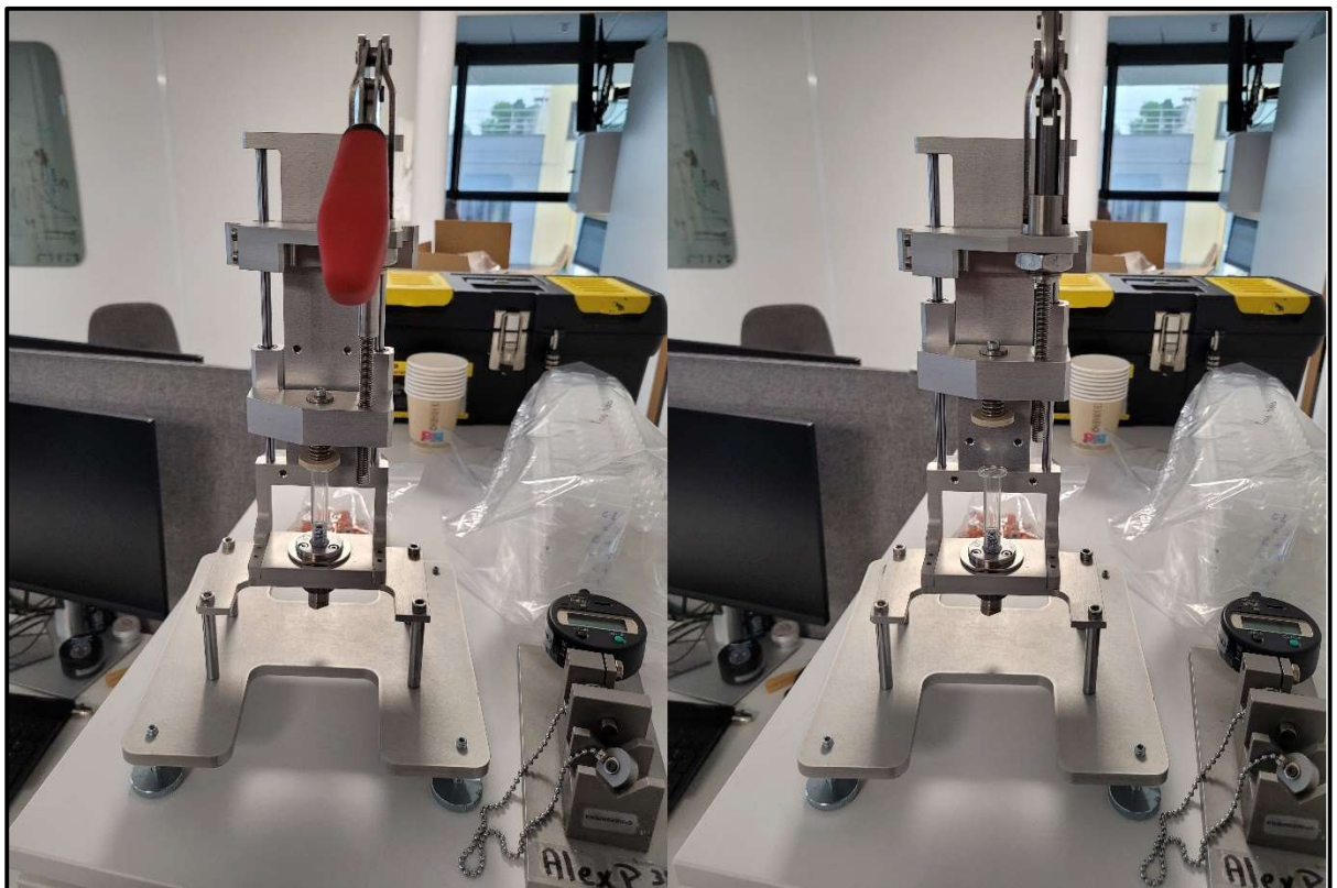
Figure 29 : Tool to assemble PRTC and barrel.
