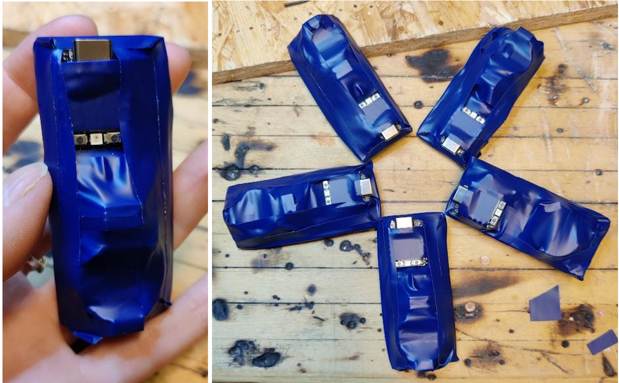
Figure 18. Soldered protoboards covered in electrical tape
