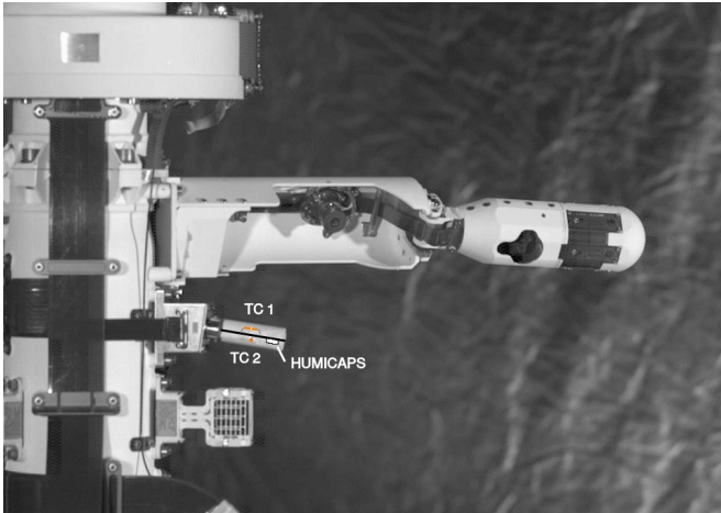
Figure 2.4. MEDA HS mounted on the Remote Sensing Mast of Perseverance. The Figure indicates the PCB orientation inside the cylindrical shield, and the locations of the HUMICAP heads (capacitive humidity sensors that include also platinum resistance thermometers) and the THERMOCAP sensors used to measure PCB temperature. Credit: NASA/JPL-Caltech, adapted by the author.
