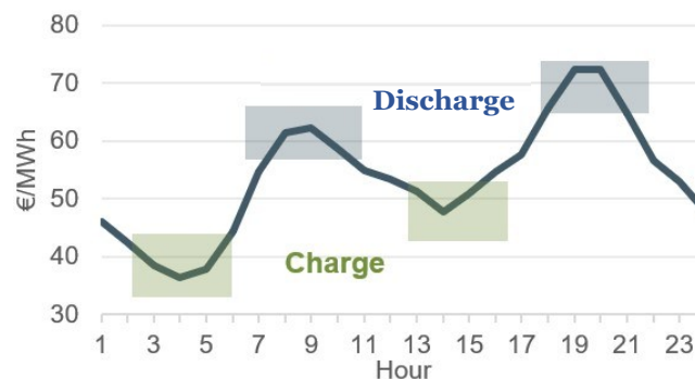
Figure 33, Principle of energy arbitrage (ECA 2021)
