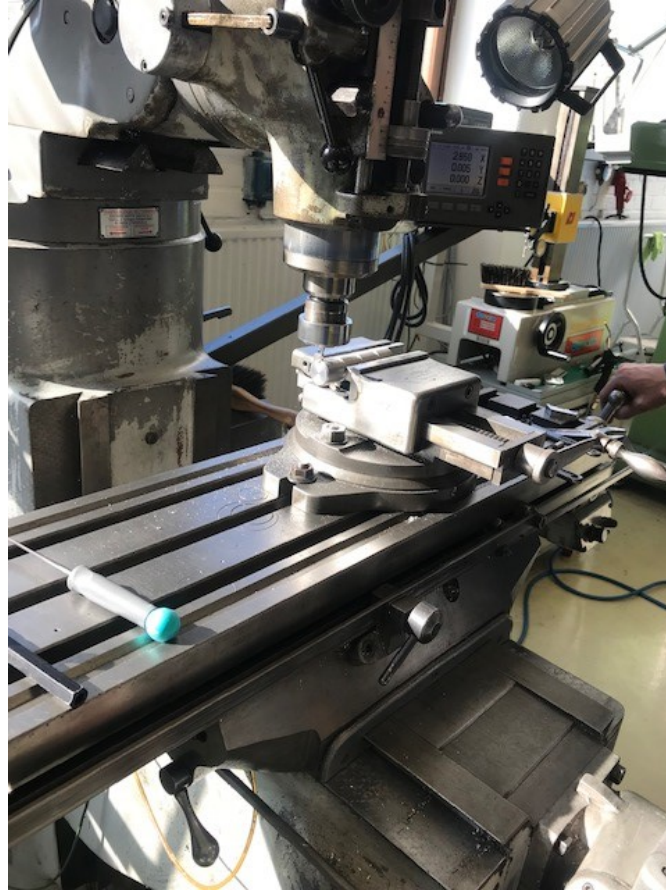
Figure 12. Keyway Milling Process.
