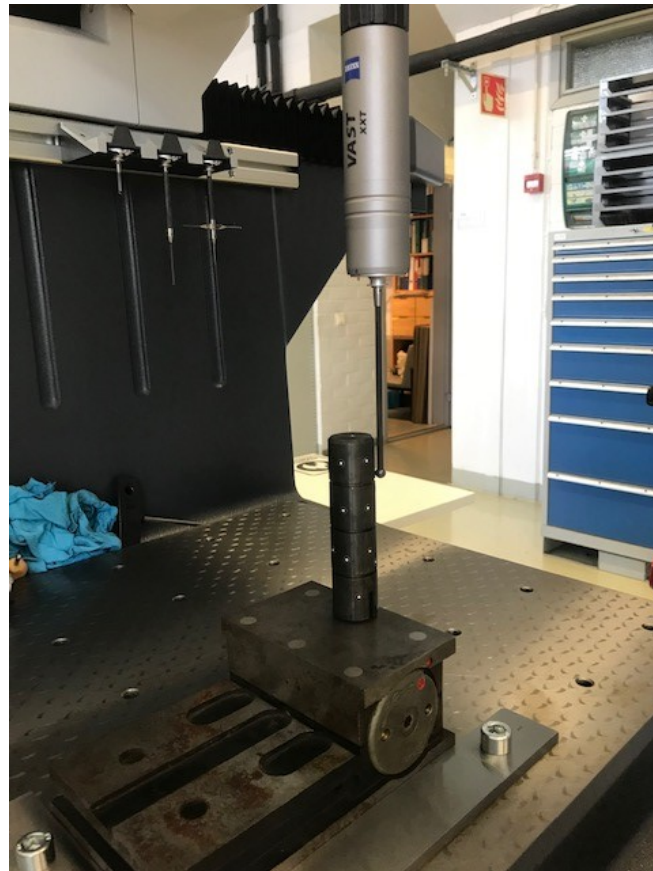
Figure 32. Zeiss CMM Inspection of The Tolerance Bar.
