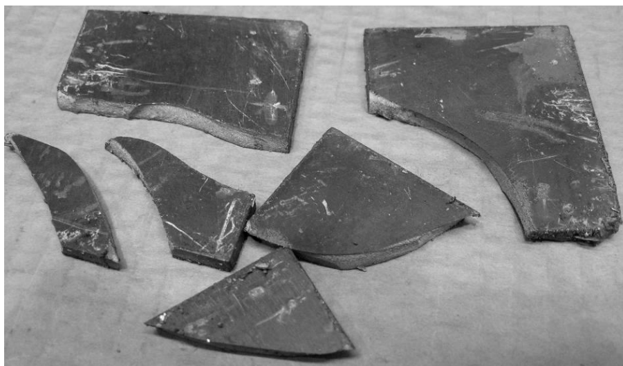
Figure 11: Pieces of two hammered Nd-Fe-B magnets.
