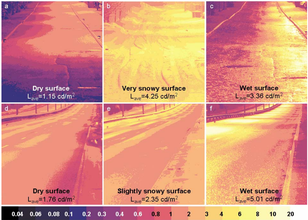
Figure 6. Luminance measurement results from a local street in Espoo, Finland, illuminated by HPS lamps under a) dry, b) very snowy, and c) wet weather conditions. Luminance measurement results from Highway 3 in Helsinki, Finland, illuminated by HPS lamps under d) dry, e) slightly snowy, and f) wet weather conditions (Ekrias et al 2007).
