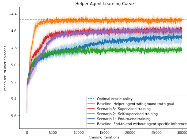
Figure 6.4. Average learning curves of simulations using 8 random seeds and various helper agent architectures. The green line in the figure represents the learning curve without behavior embeddings, serving as a lower bound for the helper agent performance. The orange line displays the performance when the policy network utilizes ground truth information about the agent behavior, acting as the upper bound for helper agent performance. The blue line represents end-to-end training with embeddings (scenario 1), the purple line corresponds to action prediction pre-training (scenario 2), and the red line indicates goal prediction pre-training (scenario 3). The shaded region illustrates the standard deviation over 8 seeds.
