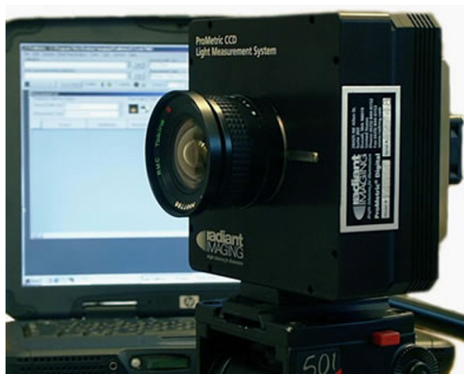
Fig. 3. The imaging luminance photometer ProMetric 1400.
