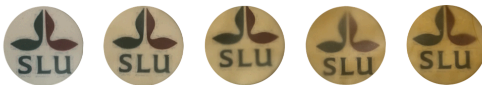
Fig. 1. Aspect of the films. From left to right: CNF, CNF/LCNF 25, CNF/LCNF 50, CNF/LCNF 75, LCNF.
