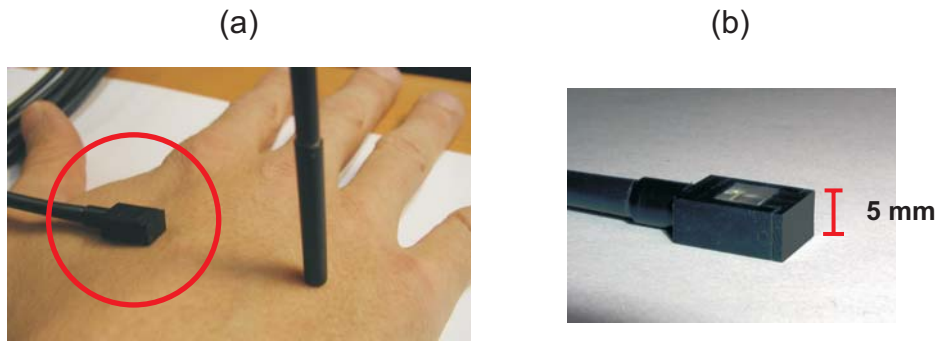
Figure 3.6: a) Photograph of prism (circled) and cylindrical terminals of fibers. b) Close-up picture of the prism terminal with one of the faces pointing upwards.
