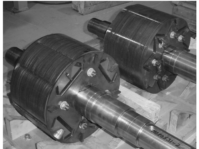
Fig. 15. Rotor stacks without magnets.
