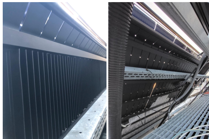
Figure 7: Left) The back of the finned PVT with the vertical fins visible. Right) Back of the non-finned PVT with the box-channel aluminium absorber visible.
