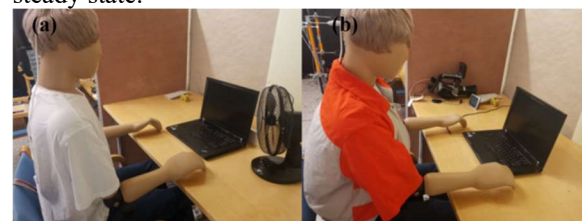
Fig. 2. Thermal manikin test with (a) table fan and (b) air-cooled jacket. (Experiments with the evaporative cooling device fixed in the same position as the table fan were performed as well.).
