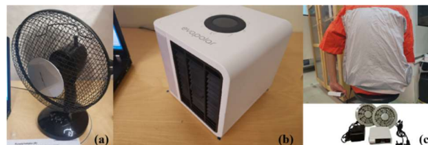
Fig. 1. Local cooling devices: (a) table fan, (b) evaporative cooling device, and (c) air-cooled jacket.
