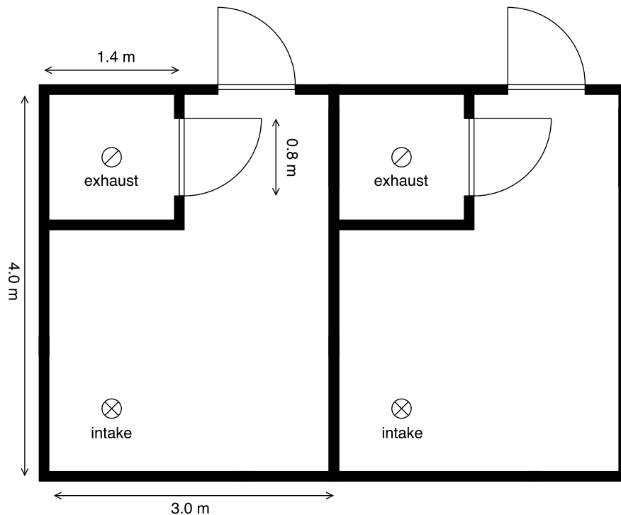
Figure 5.3: Floorplan depicting a small, two-cabin entity in one floor level connected to a singular air handling system within a passenger ship.
