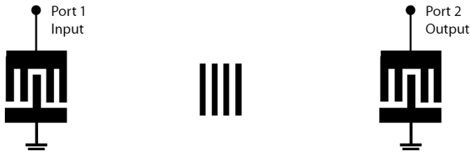
Fig. 1. Type 1 test structure. Two identical IDTs and a reflector in-between. Schematic drawing.
