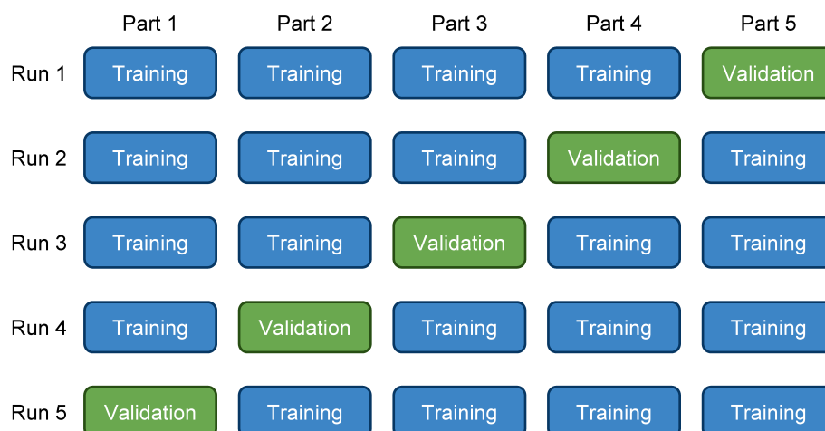
Figure 2.6: An example of 5-fold cross-validation and how the five different parts are used for training and validation during the different runs.
