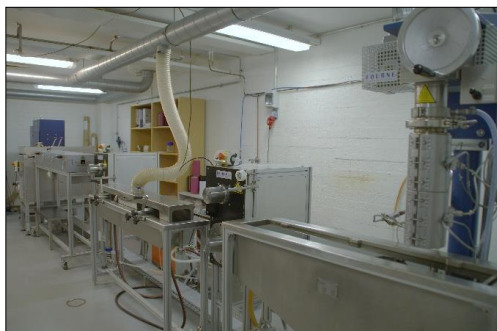
Figure 4.14. Dry-jet wet spinning unit at Aalto University.
