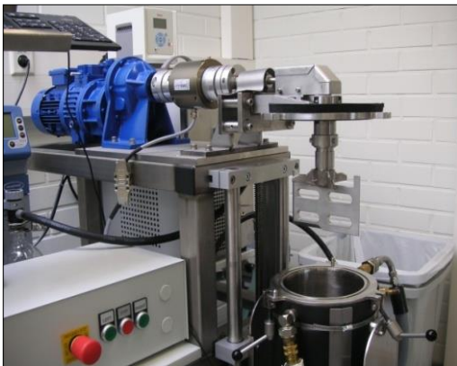
Figure 4.8. Vertical kneader for cellulose dissolution.
