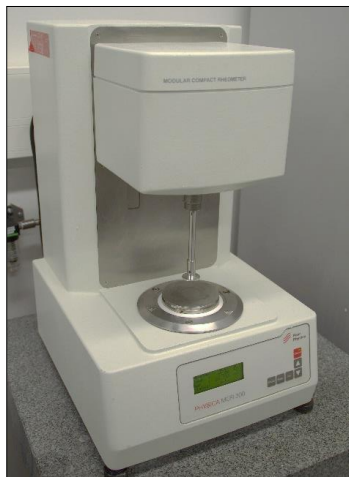
Figure 4.10. Anton Paar MCR 300 with plate-plate geometry. Above: sample loaded between the two plates.
