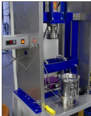
Figure 4.9. Hydraulic pressure filtration unit.
