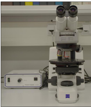
Figure 4.17. Zeiss Axio Scope polarized microscope equipped with a 5\lambda Berek compensator.
