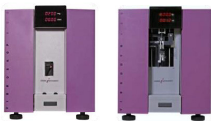
Figure 4.16. Lenzing instrument vibroskop (left) and vibrodyn (right).
