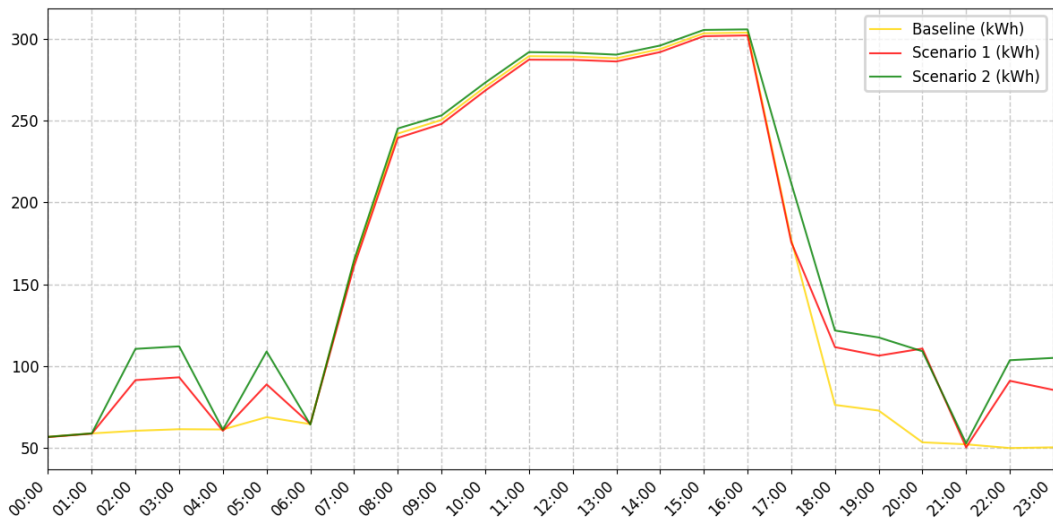
Figure 15. The net impact of four individual demand response events, measured across the entire day (10 th of June 2023). The reserve market presented in the figure is mFRR energy market (downregulation).
