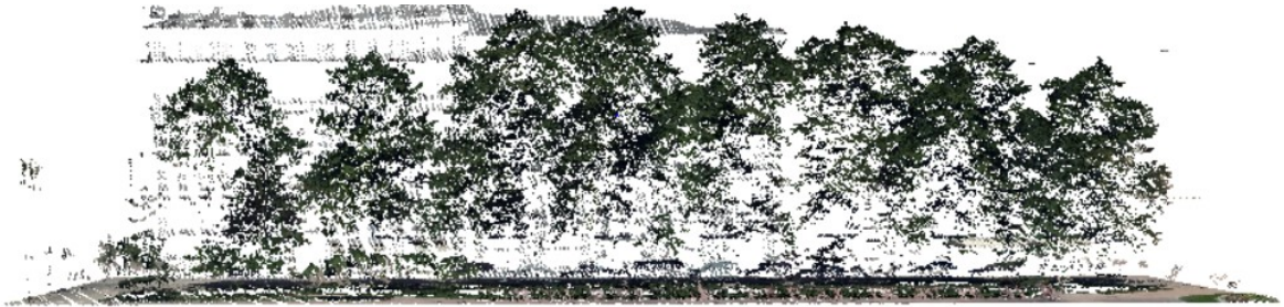
Figure 18 A side view of the laser data. Each laser point has been given an RGB value from aerial images.
