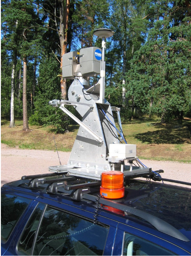
Figure 3 A mobile laser scanner on top of a car (Holopainen et al. 2013a, ©Antero Kukko)
