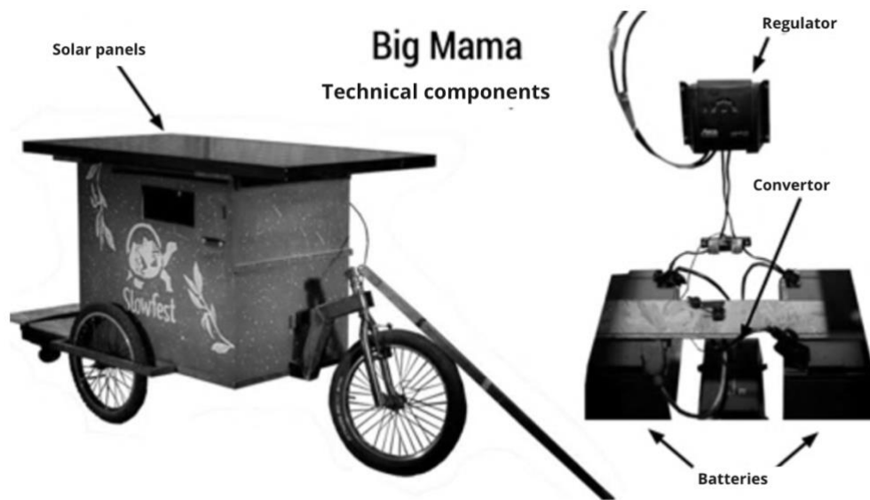
Figure 17: Technical component image of the Big Mama (250 persons capacity) Source: https://SlowFest.org/
