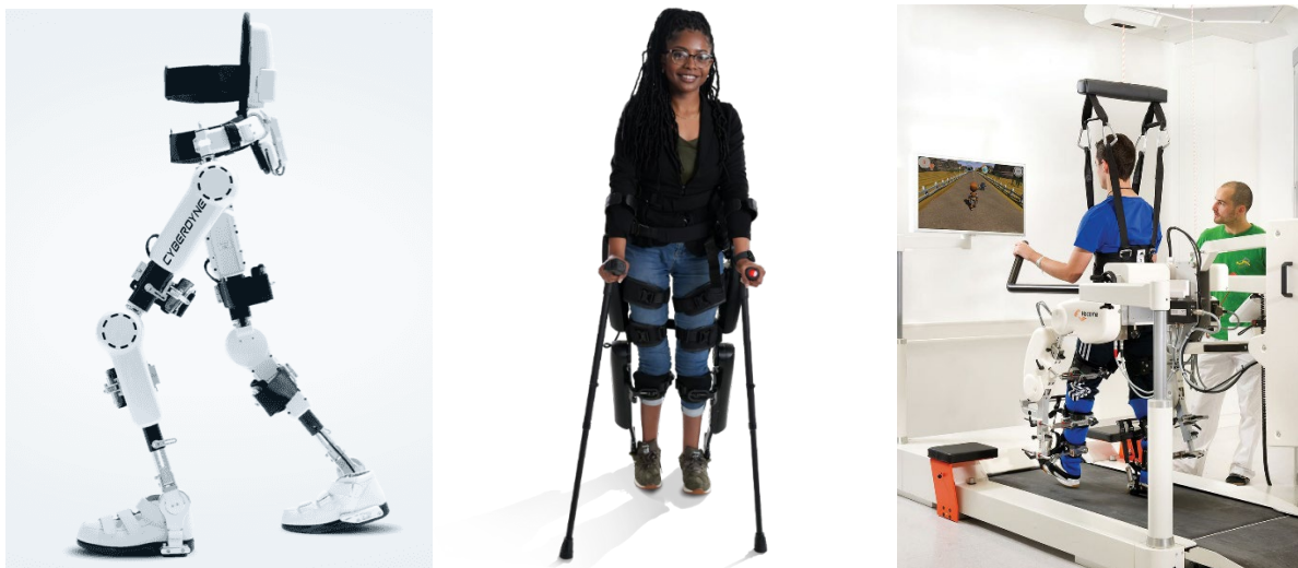
Figure 3-1. On the left side HAL lower-limb (HAL-ML05) exoskeleton [29], in the middle ReWalk 7 exoskeleton [30], and on the right side a treadmill Lokomat exoskeleton [31].
