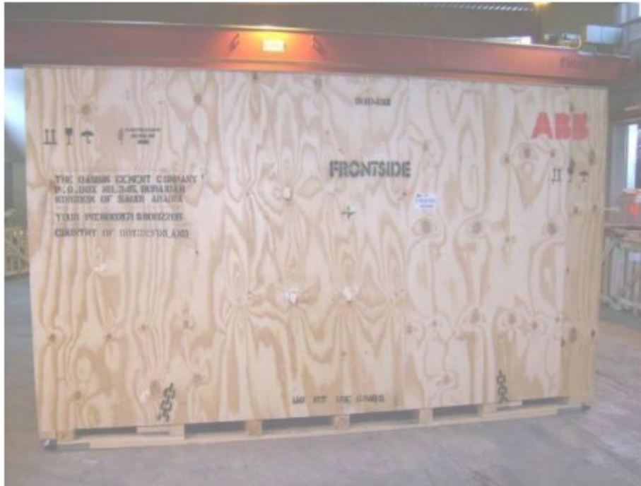
Figure 24. (Otava, 2021) Seaworthy package according to the ABB Marine packaging instructions
