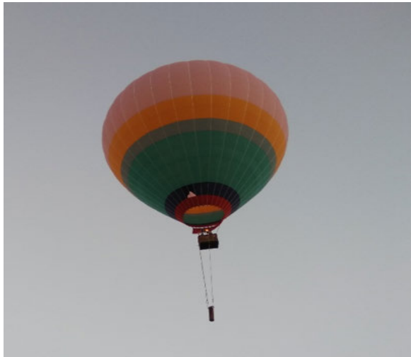
(a) Precision airdrop system by hot-air balloon
