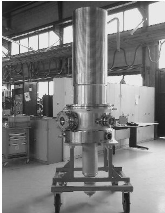
FIGURE 1.1. 140 GHz prototype gyrotron for W7-X (fabricated by Thales Electron Devices, Vélizy). [33]
