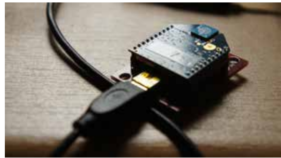
Fig. 4.2.4 Accelerometer attached to the kite. Arduino FIO + Xbee
