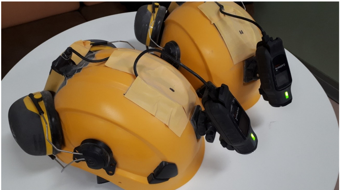
Figure 6: The camera system on workers' helmets during the video recordings
