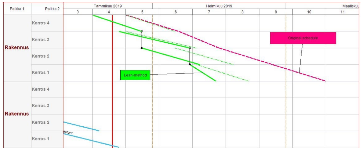
Figure 24: Schedule projection of building C comparing the original and improved methods
