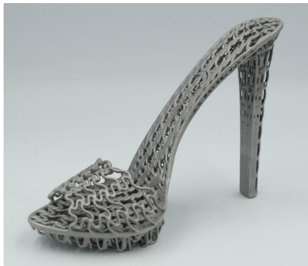
Figure 1. AM aluminium part (Manufacturer: FIT AG, Germany)
