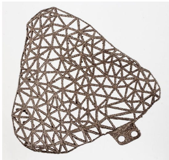
Figure 11. AM titanium implant structure (Photo: M.Sc. (Tech.) Pekka Paavola)
