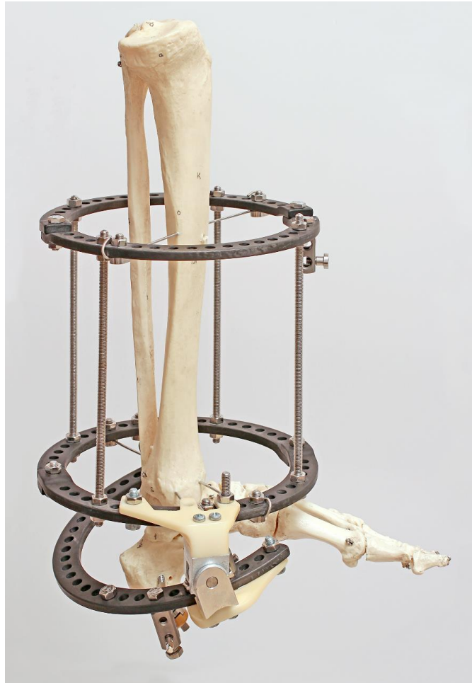
Figure 6. Patient-specific ankle-support device, in which white AM parts are custom made according to measured ankle movements. (Photo: M.Sc. (Tech.) Pekka Paavola)
