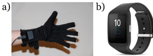
Figure 8. Hand/arm-worn devices. a) Data glove (5DT-5 Ultra). b) Smartwatch (Sony SmartWatch 3 SWR50, source: https://www.sonymobile.com/global-en/products/smart-products/smartwatch-3-swr50/#black , downloaded 22 Nov 2017, with permission).
