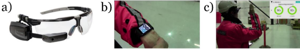
Figure 15. Devices for the wearable maintenance in Study II. a) Vuzix M100 smart glasses (image courtesy of Vuzix Corporation). The image is displayed in the small screen shown on the black piece over the bottom part of the right lens. b) The smart watch. c) A user using hand gestures to change the information shown in the smart glasses (upper right corner).
