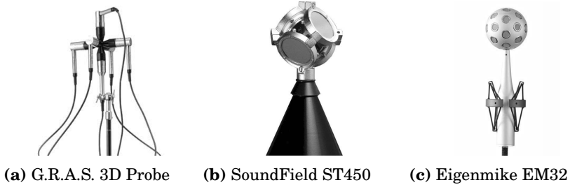
Figure 2.3. Different commercially available spherical microphone arrays, utilized in different publications in this thesis.
