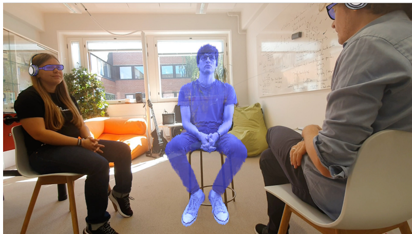
Figure 1.1. Concept of an AR telepresence meeting. Two participants are in a room, while a third remote-end participant is rendered using head-mounted displays (HMDs) and headphones.
