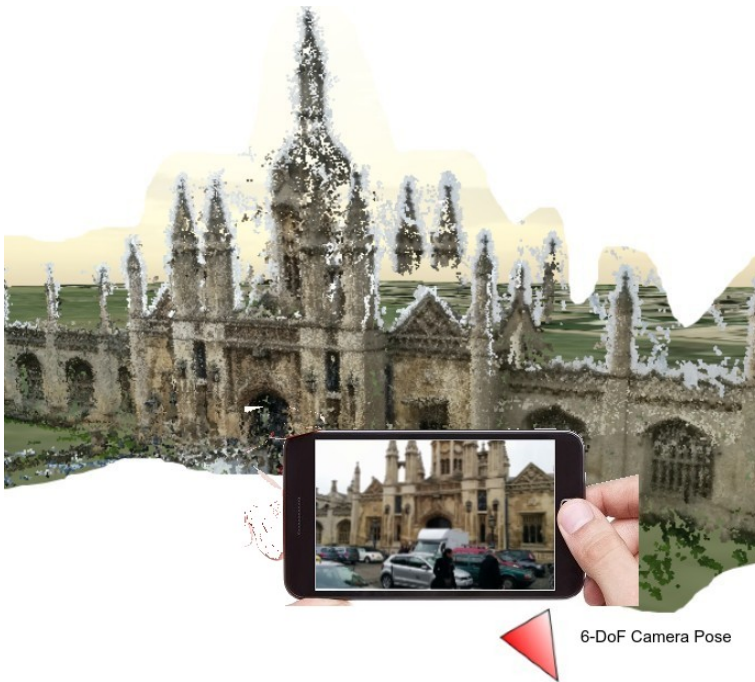
Figure 4.1. Image-based localization aims to recover the 6 DoF camera pose w.r.t to an environment [57] from an input image (e.g. captured by a mobile phone camera). The environment is represented as a 3D point cloud or a database of images with respective poses and local 2D keypoint representations.
