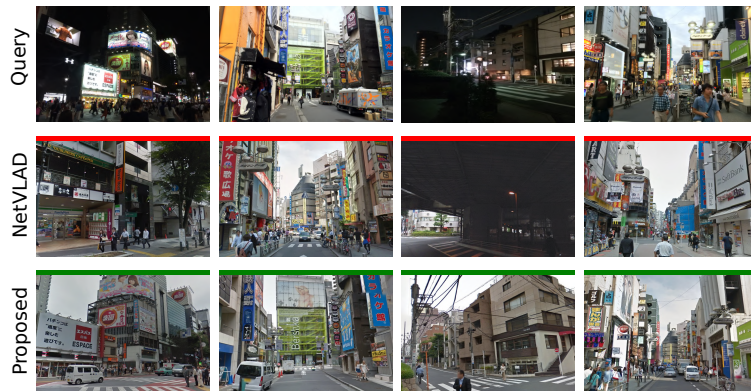
Figure 3.2. Qualitative results produced by Publication IV on Tokyo24/7. Each column corresponds to a query, and the top-1 NN database images by NetVLAD [5] and the verification method proposed in Publication IV. Similarity in global properties such as geometry, illumination and viewpoint results in the failure of NetVLAD. Publication IV utilizes local similarity and geometric verification to retrieve correct database images (bottom row).
