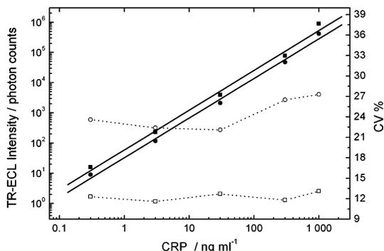
**Figure 3.** Calibration curve of the immunometric assay of hCRP with incubation times of 15 (■) and 2 (●) min and the corresponding precision profiles presented with dotted lines with incubation times of 15 (□) and 2 (○) min. For details, see the Experimental Section.
