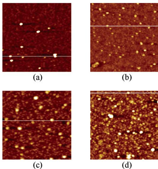
**Figure 2.** Surface structure of a silicon electrode in different stages of the ECLIA process as monitored by AFM. Conditions: all image sizes  $1 \times 1 \mu\text{m}^2$ , (a) natural oxide film on the Si electrode measured after cutting silicon wafers into the pieces without any other treatment, (b) Si electrode covered with  $\sim 4$ -nm-thick thermal oxide film, (c) Si electrode coated with primary anti-hCRP antibodies, and (d) coated and saturated Si electrode.
