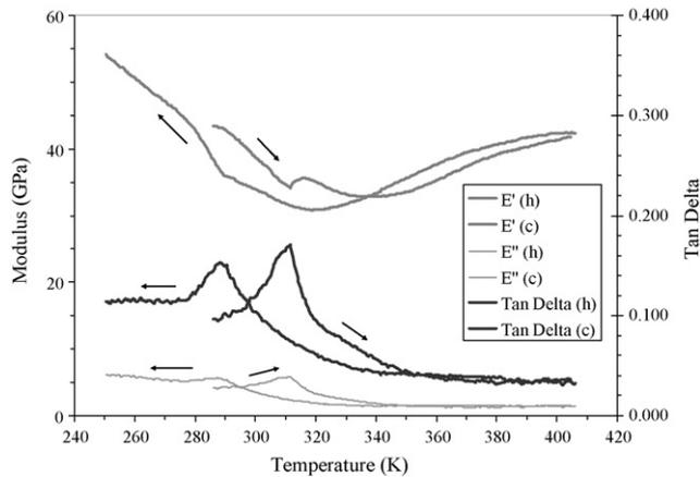
Fig. 1. DMA measurement curves of the sample A1 as a function of temperature.
