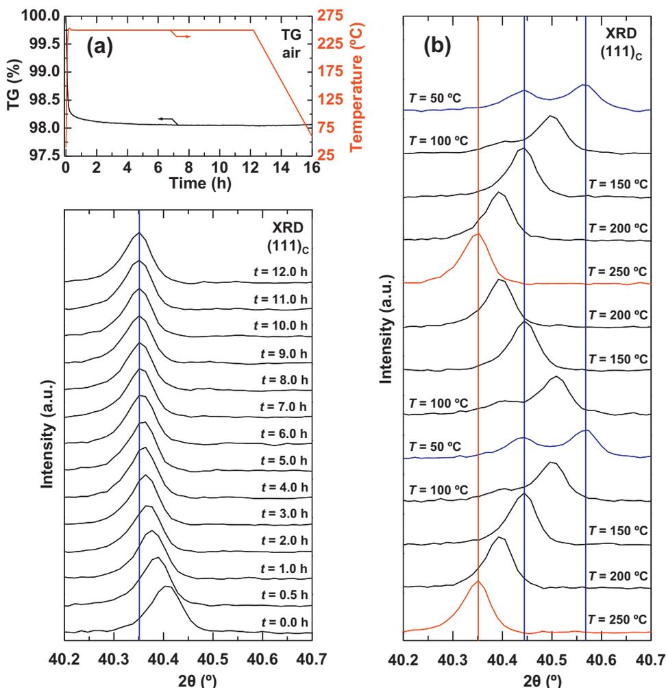
**Fig. 2.** (a) Oxygen deintercalation from  $\text{SrCoO}_{3-\delta}$  precursor phase (at 250 °C, 1 atm stagnant air) as seen through weight reduction in TG analysis (upper panel) and negative  $2\theta$  shift in in situ XRD patterns (lower panel). (b) Split of the pseudocubic  $(1\ 1\ 1)_C$  reflection at  $T < 150$  °C due to the separation of the two tetragonal phases T1 and T2.
