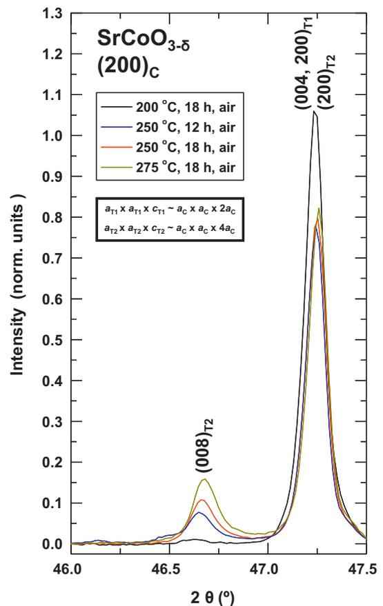
**Fig. 4.** Pseudocubic  $(2\ 0\ 0)_C$  reflections of oxygen-deintercalated  $\text{SrCoO}_{3-\delta}$  samples demonstrating the pronounced contraction of the  $c_{T2}$  lattice parameter following the increasing abundance of phase T2.
