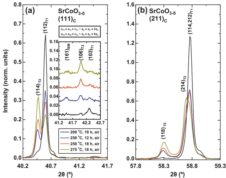
**Fig. 3.** Pseudocubic (a)  $(1\ 1\ 1)_C$  and (b)  $(2\ 1\ 1)_C$  reflections of oxygen-deintercalated  $\text{SrCoO}_{3-\delta}$  samples demonstrating the existence of two tetragonal phases, T1 and T2. (Note: The weak shoulders at  $40.8^\circ$  and  $59.0^\circ$  originate from the unfiltered part of the  $\text{Cu-K}\alpha_2$  radiation.)
