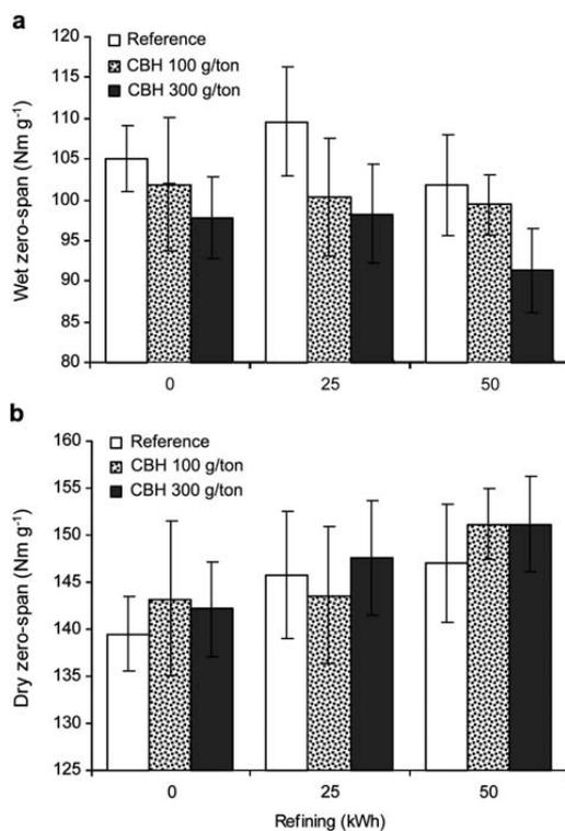
**Figure 3** Effects of CBH treatment and refining on wet (a) and dry (b) zero-span tensile indices.
