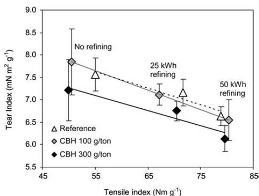
**Figure 2** Tensile and tear indices correlation.
