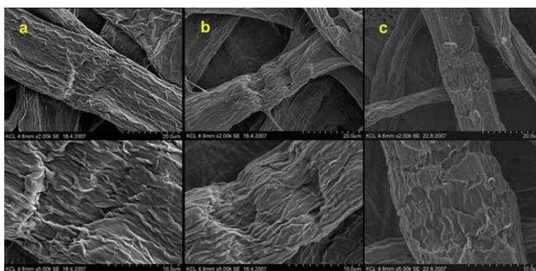
**Figure 5** SEM images of CBH treated samples: dosage – 100 (a), 300 (b), and 900 g prot. ton<sup>-1</sup> (c); magnification: 2000 $\times$  (top) and 5000 $\times$  (bottom).
