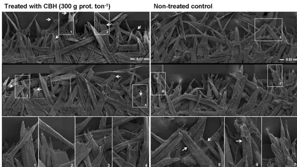
**Figure 4** SEM images from the rupture zone of wet zero-span testing. Left: CBH (300 g prot. ton<sup>-1</sup>) treated sample. Arrows indicate fibers with clean, straight fractures, hypothetically ascribed to the impact of CBH. Right: Non-treated control sample. Arrows indicate examples of fracture type predominant in control sample. In both cases, frames in the image represent magnified areas depicted in the lower part of the Figure.
