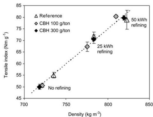
**Figure 1** Tensile index vs. apparent density relationship for control and CBH treated pulp.
