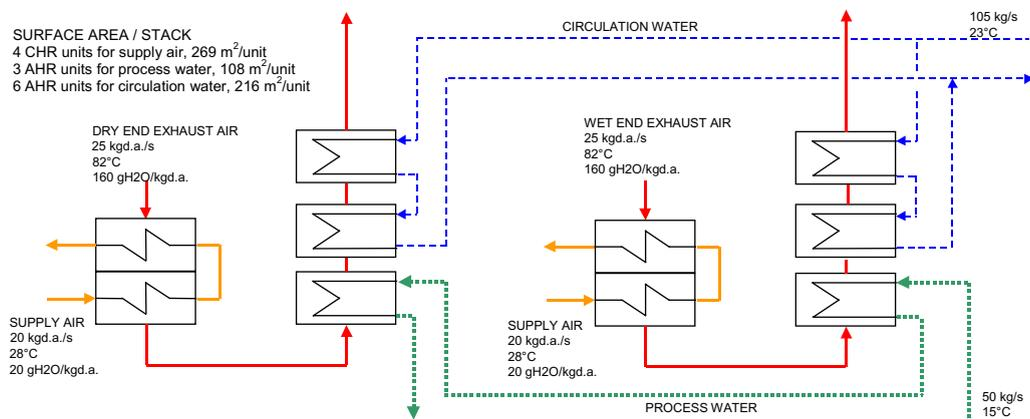
Fig. 5. Example heat recovery system with two heat recovery stacks.
