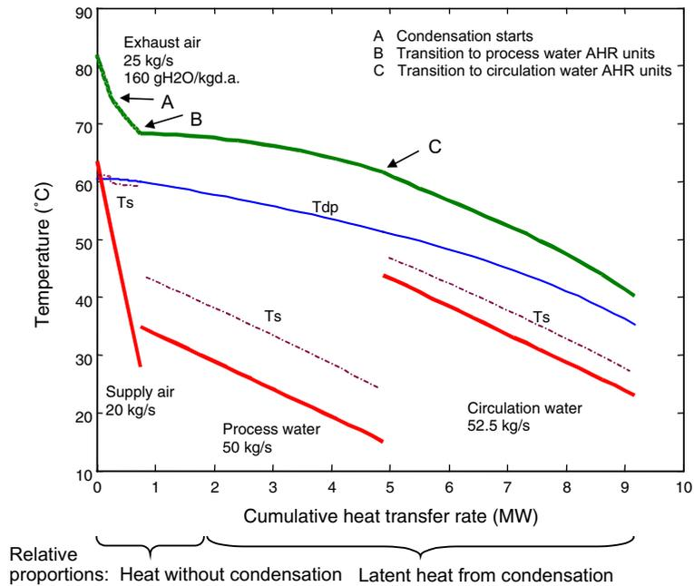
Fig. 3. Heat transfer in the example heat recovery stack with design values.
