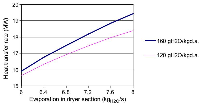
Fig. 6. Total heat transfer rate with two different humidities of exhaust air in the example heat recovery system.
