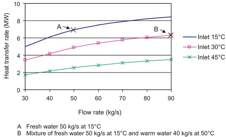
Fig. 8. Heat transfer rate in relation to the flow rate and inlet temperature of process water in the process water AHR units of the example heat recovery system.
