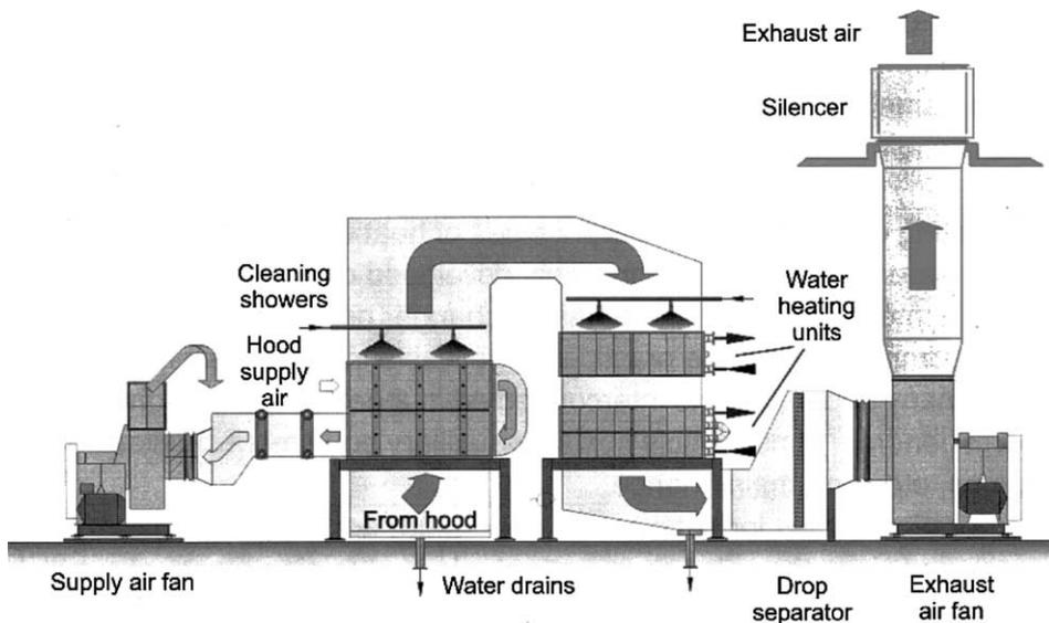
Fig. 1. Modern heat recovery system of paper machine dryer section [1].
