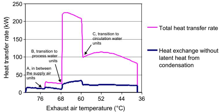
Fig. 4. Heat transfer rate in the example stack divided into heat transfer without condensation and total heat transfer rate.
