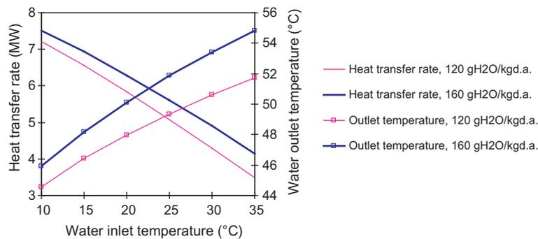
Fig. 7. Heat transfer rate and water outlet temperature in relation to water inlet temperature in the process water AHR units of the example heat recovery system.
