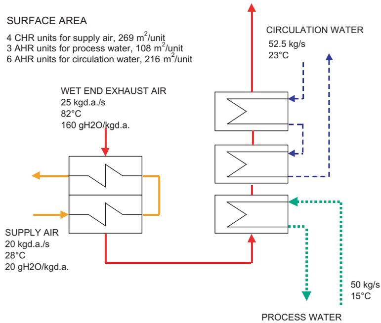
Fig. 2. Structure of an example heat recovery stack. The abbreviation d.a. refers to dry air.
