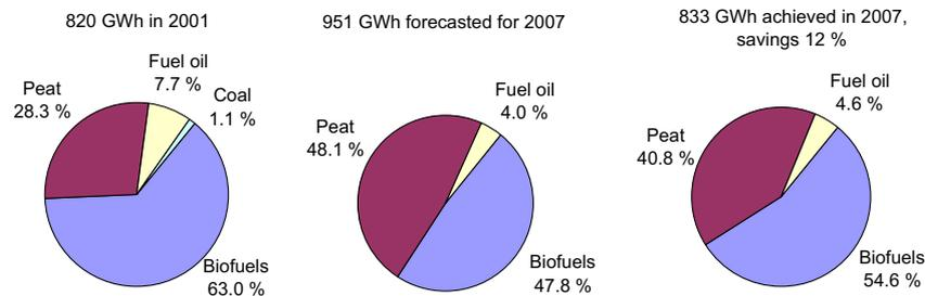
Fig. 5. Fuel use in 2001 and the forecast and actual fuel uses in the case mill in 2007.
