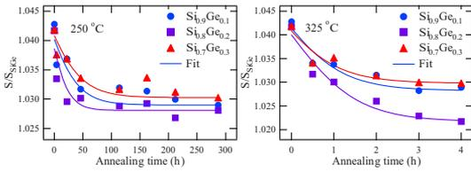
FIG. 1. (Color online) Measured (markers) and fitted (lines) low-momentum parameter  $S$  as a function of annealing time in samples annealed at 250 °C (left panel) and 325 °C (right panel). Points at  $t=0$  correspond to “as-irradiated” values associated with  $E$  centers.
