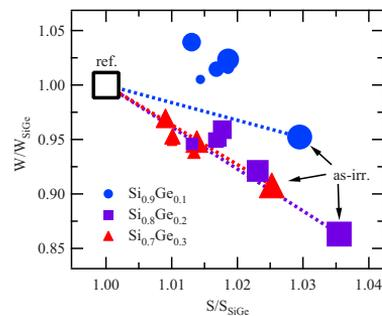
FIG. 3. (Color online) The  $(S, W)$  parameters measured in irradiated and annealed  $Si_{1-x}Ge_x$  layers. The data shown are the final points from each annealing series. The decrease in symbol size visualizes increasing annealing temperature.
